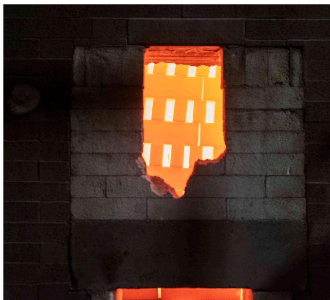
Photo 1: Clay units visible during firing process through an opening in a tunnel kiln
